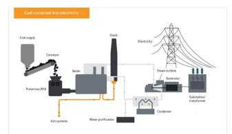
**Figure 1** The pulverized coal combustion (PCC) system uses to convert coal to electricity. Adapted from World Coal Association. Copyright 2013 by VGB Power Tech.
