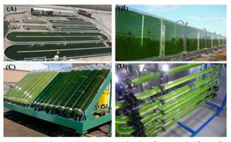
**Figure 5** The Algae cultivation methods. A) Natural, B) Artificial (flat plate photobioreactor), C) Tubular photobioreactor and D) Column photobioreactor (Adeniyi et al., 2018)
