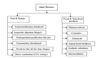
Figure 4 The flow chart of algae biomass production (Adeniyi et al., 2018)
