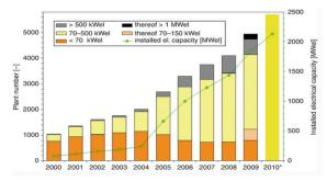
Figure 3 Biogas for electricity generation in Germany. (Scholwin and Nelles, 2013)
