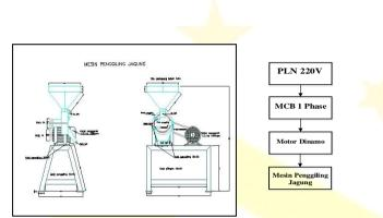
This electric motor driven corn kernel crushing machine is designed using fairly simple materials at an affordable price. In this corn kernel grinding machine, the author made a final project that designed all parts of the tool and its components.
