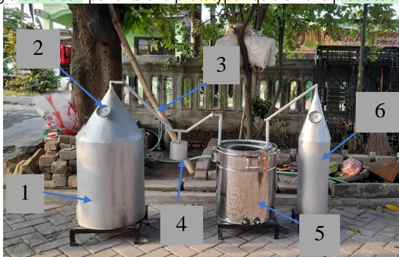
Figure 2 : Results of making a prototype liquid smoke production tool
