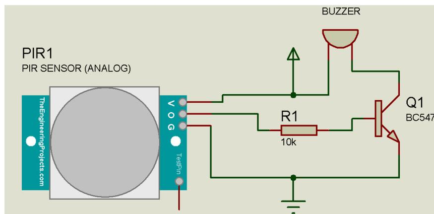
Figure 3. PIR schematic circuit
