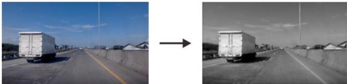
Figure 7. Conversion of RGB to Grayscale
