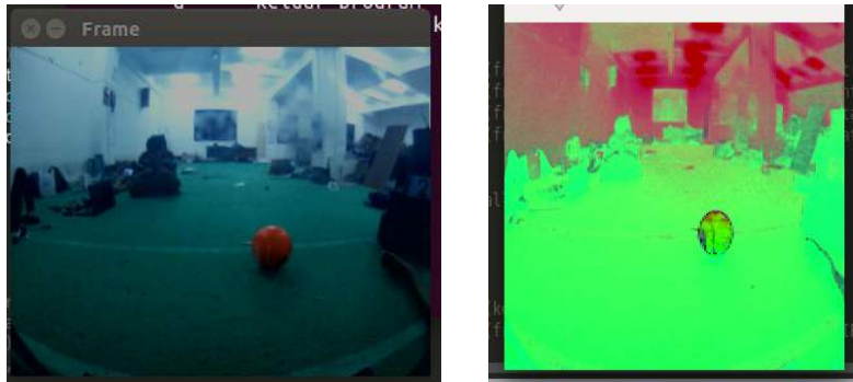
Figure 8. (a) Frame with RGB (b) HSV conversion results
