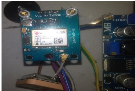
Figure 8. GPS Ublox Neo Not Blinking
